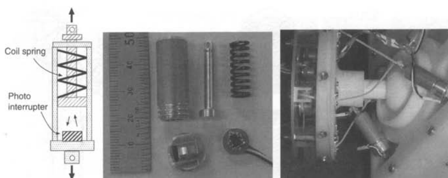
Fig. 9. Left: tension sensor unit with a photo interrupter, Right: crotch joint
