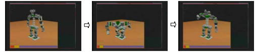
Fig. 5: Apply the optimized pick-up motion-capture data to the robot "Cla" after learning
