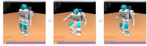
Fig. 4: Apply the optimized pick-up motion-capture data to the robot "Hoap" after learning
