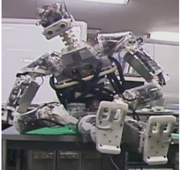
Figure 1: Kenta: a whole-body tendon-driven flexible-spine humanoid
